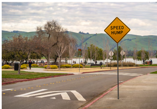
Figure 24. Traffic Calming Devices
